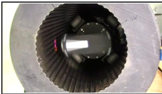
BEMIS-LC™ Scanning 155mm Gun Tube
